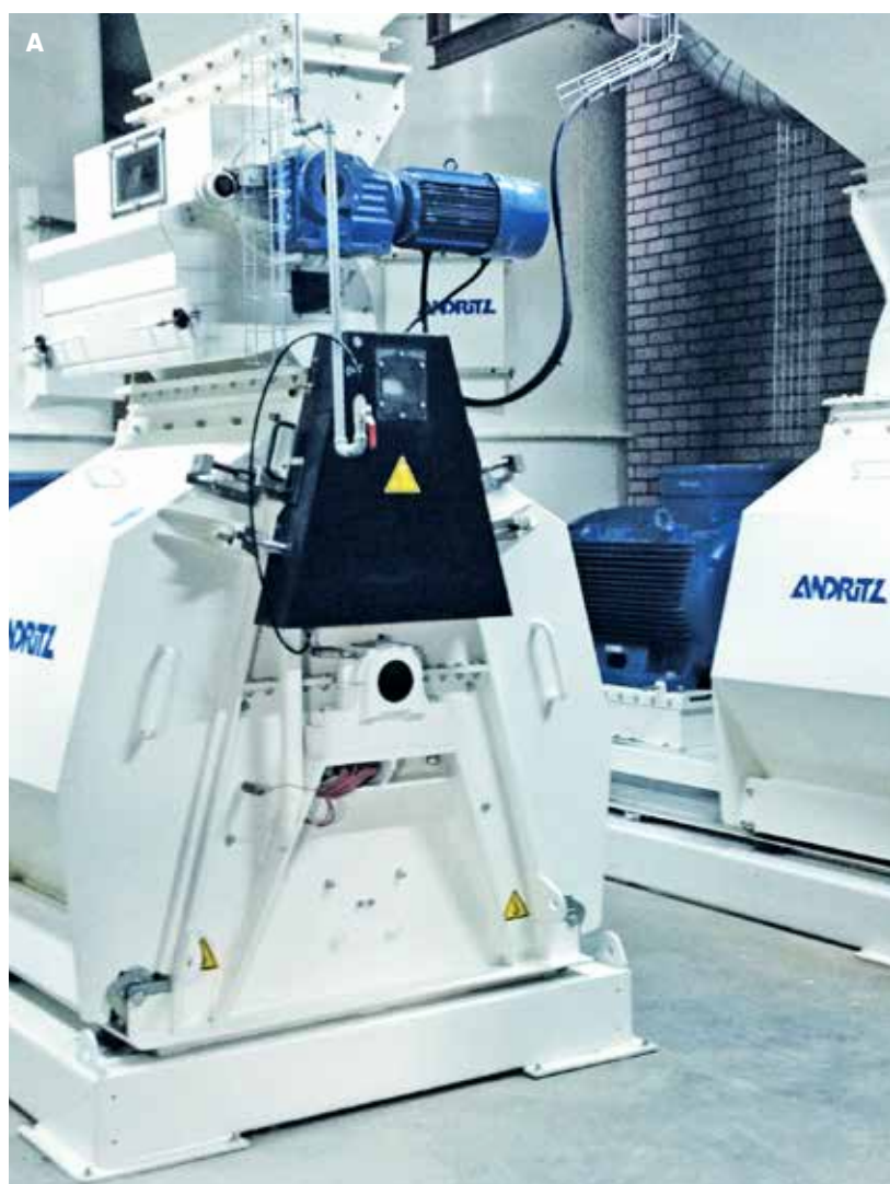
A The Optimill consists of a hammer mill for raw material grinding of normal to coarse structured feed products, such as cattle, pig and poultry feeds.
