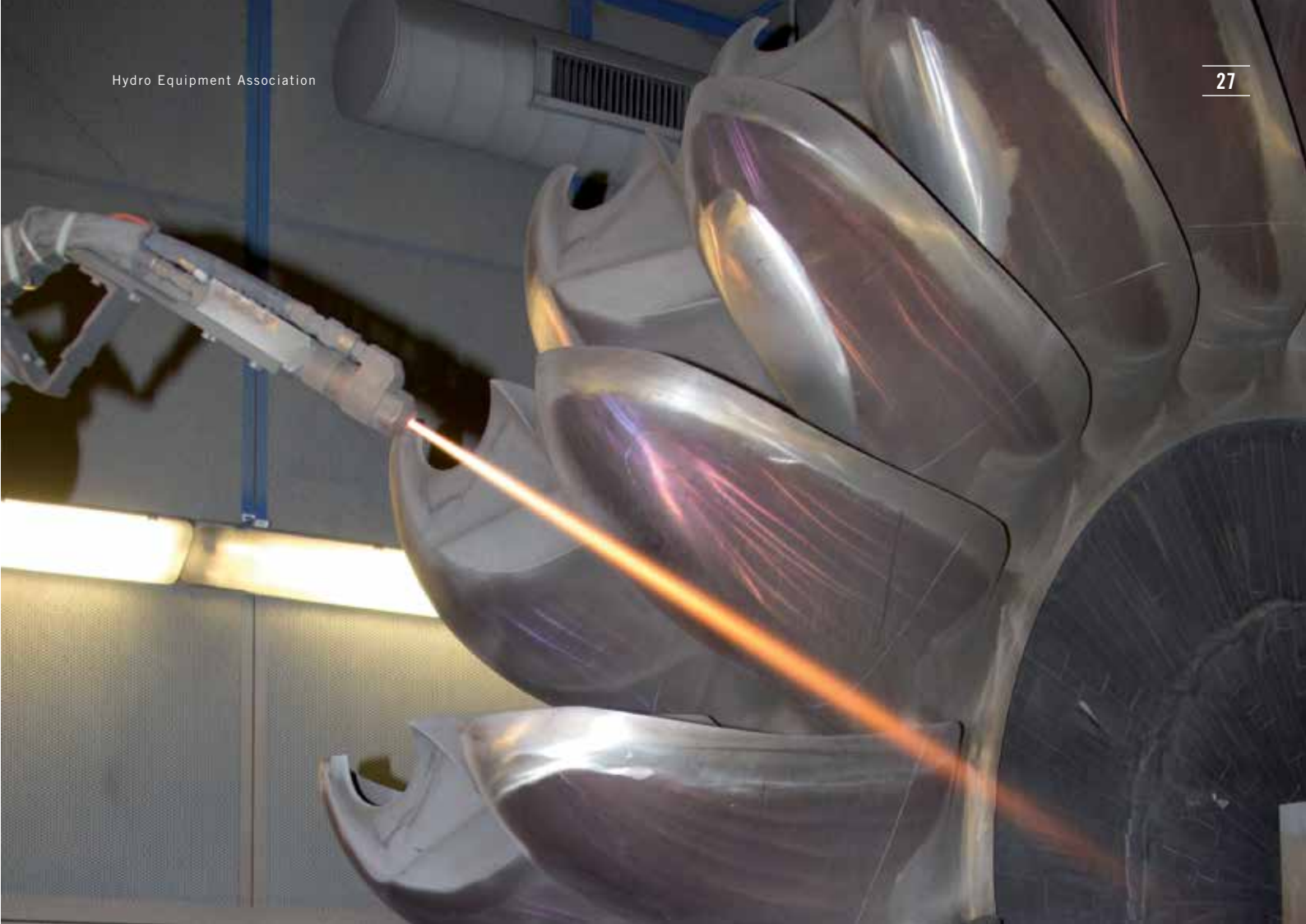
Figure 15: Coating of a Pelton runner using the high velocity oxyfuel process (HVOF). The average thickness of the coating is 0.3 mm.
