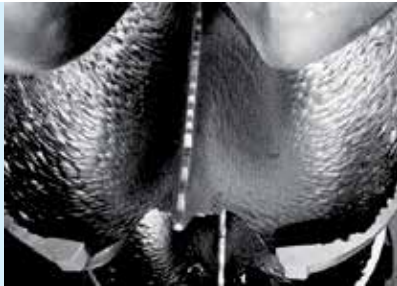
Uncoated Pelton runner after 38,000 t of particles have passed through the turbine.
