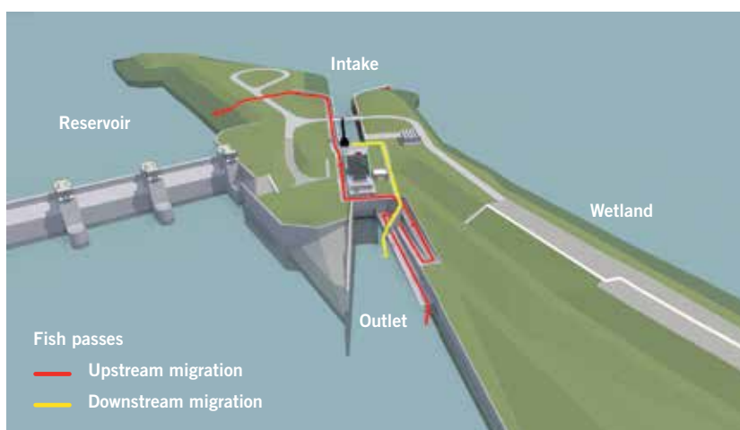
Figure 36: Diagram of Rocheмаure small hydropower plant. The upstream passage consists of 50 pools, the downstream passage (designed with the needs of eels in mind) of a 190 m 2 fine screen (2 cm gap between bars) at an angle of 20° to the flow. The screen guides the fish up to the passage entrance without crushing them against the flow. The plant (both its power generation and fish passage parts) was designed by CNR, which also supplied this picture.
