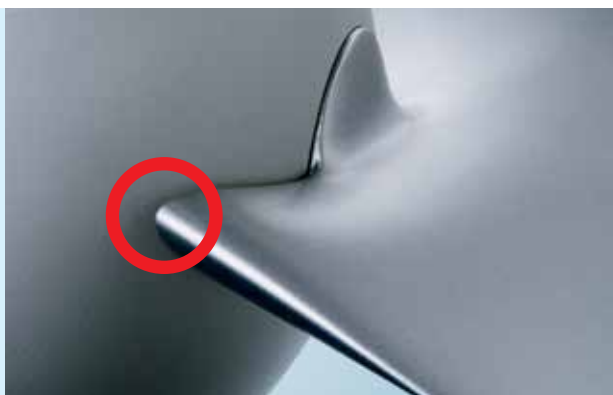
Figure 34 a: Minimum gap runner Kaplan turbines increase fish survival rates by making the gaps between blade and hub and blade and periphery as small as possible. Compare image on the left (minimal gap of trailing blade edge) with that on the right (wider gap).
