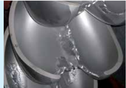
Pelton runner with latest coating technology after 183,000 t of particles have passed through the turbine.
