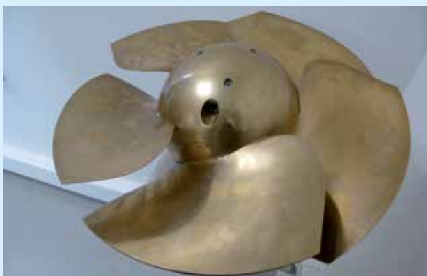
Figure 34 b: The minimum gap runner viewed from an angle revealing its spherical turbine head (a design feature that increases fish survival).
