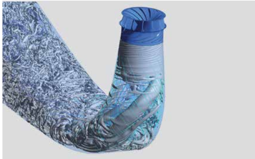
Figure 9: Simulation of turbulent sub-structures downstream of a Francis turbine
