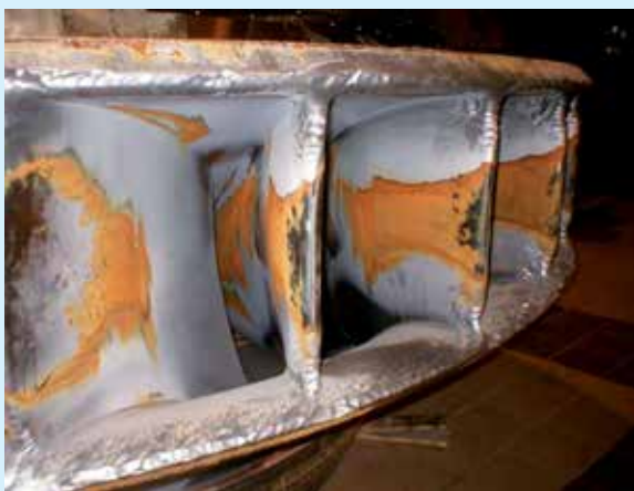
Figure 17: The possible extent hydro-abrasive erosion was not known at the time the runner on the left was installed at the Nathpa Jhakri plant, India. Its only protection against erosion was a desander. It was replaced by a runner designed to be fully coated by robot. The runner for the power plant upstream (Karcham Wangtoo, right) was designed with the same requirement in mind, and additionally for ease of replacement, by allowing the generator to remain in place.
