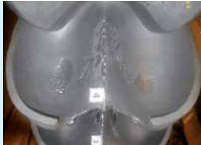
Pelton runner with standard coating after 120,000 t of particles have passed through the turbine.
