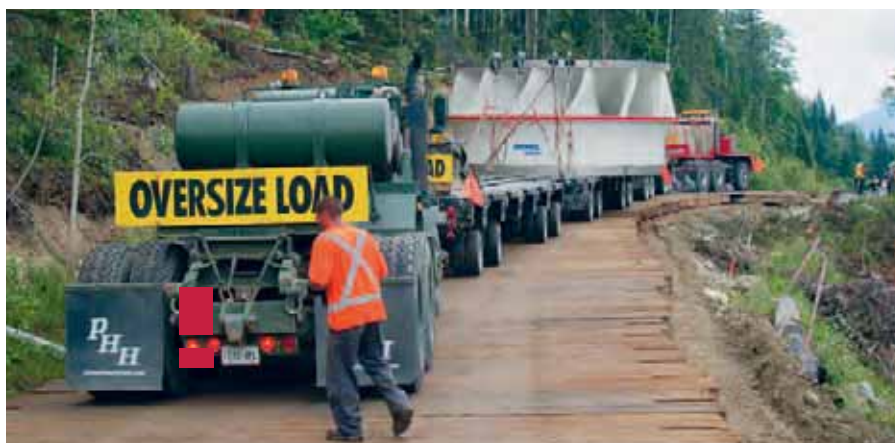
▣ Delivery of 520 MW runner for unit #5 at HPP Mica in British Columbia
