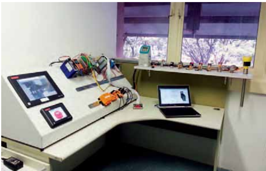
Mobile bench for training of ASi network and bench of instruments for supporting to the field
