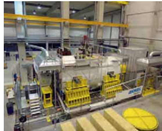
Hydrogen-cooled turbogenerator in test field
