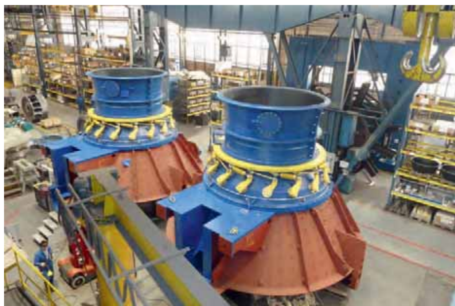
▣ Compact Axial Bulb turbines for HPP Lixhe during workshop assembly
