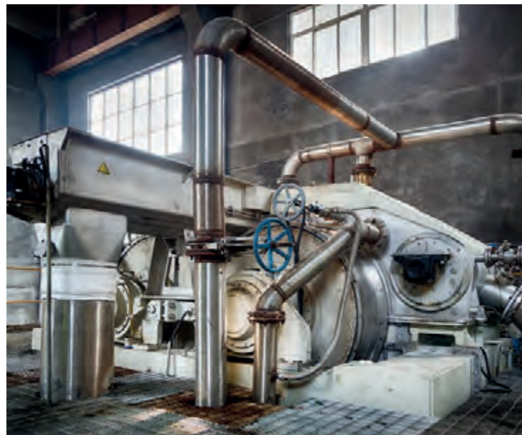
◀ The ANDRITZ Wash Press (AWP) is the first in China. The compact unit performs P-stage bleach washing in the dissolving pulp process.
