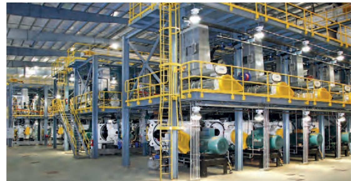
◀ Georgia Biomass operates 22 large ANDRITZ pellet mills to produce 750,000 t/a of pellets.
