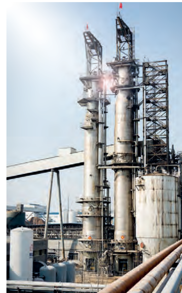
◀ The ANDRITZ PHV (Pre-Hydrolysis Vessel) is a new technology developed for hemicellulose removal with continuous cooking. The world's first PHV was delivered to Sun Paper and is shown here next to the existing continuous cooking system. The mill has the flexibility to swing production between dissolving and traditional kraft pulp.
