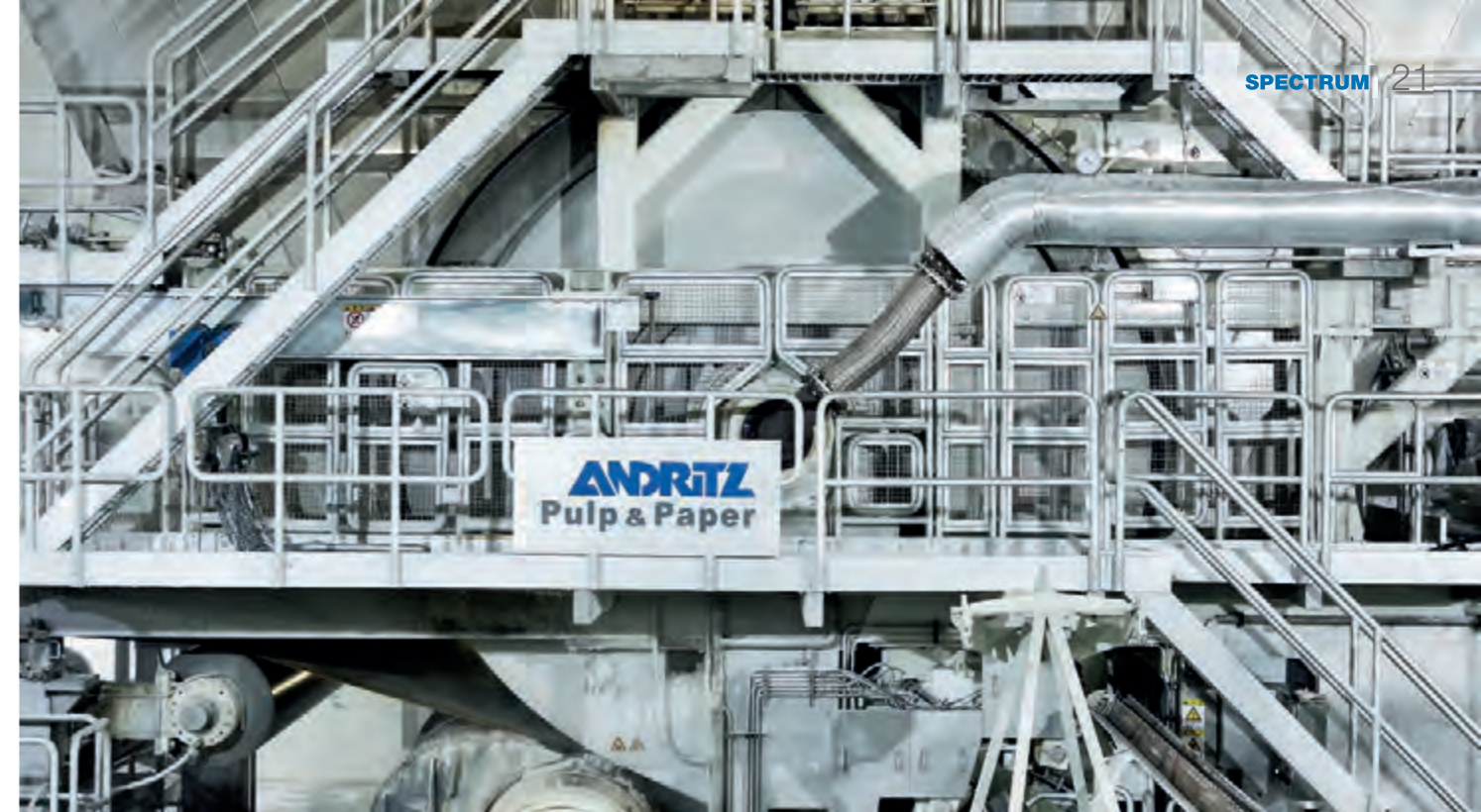
▲ The heart of the Hengan machine: an 18 ft. diameter PrimeDry Steel Yankee.
