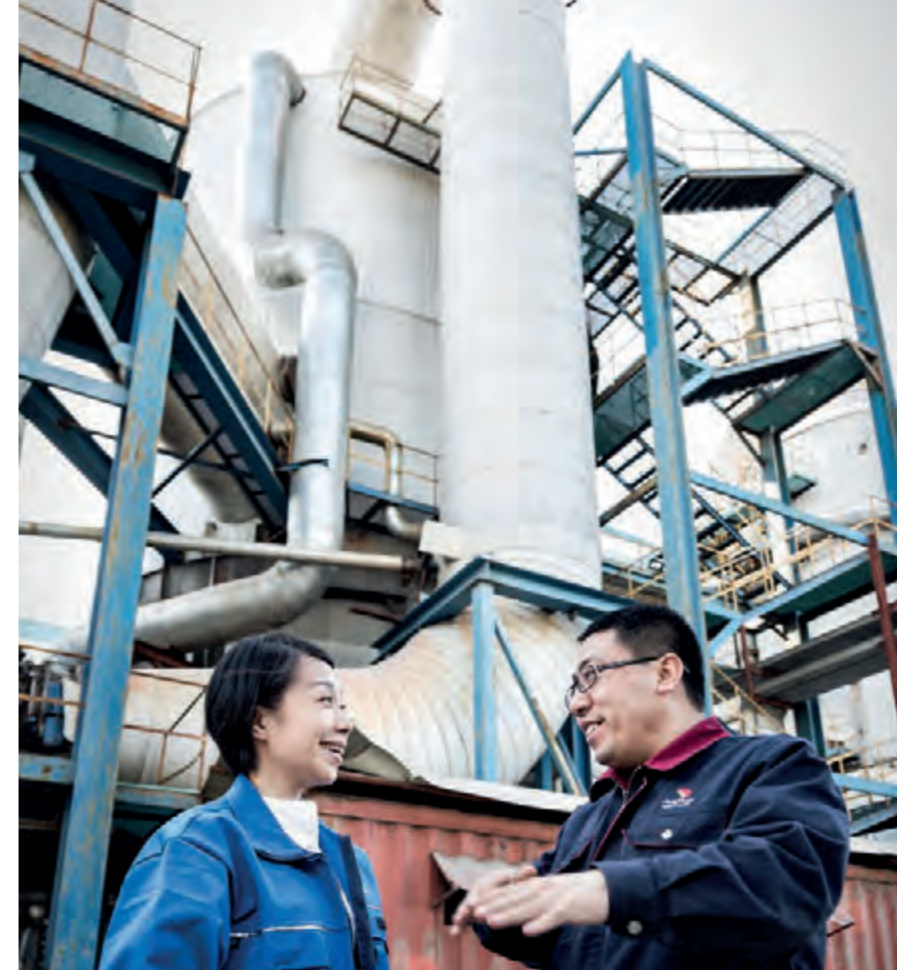
◀ Chen Jieyu of ANDRITZ (left) with An Qingchen of Sun Paper in front of the ANDRITZ MVR evaporators which considerably reduce fresh water consumption in the mechanical pulping lines. Sun Paper is leading the world with its zero discharge accomplishments at this mill.
