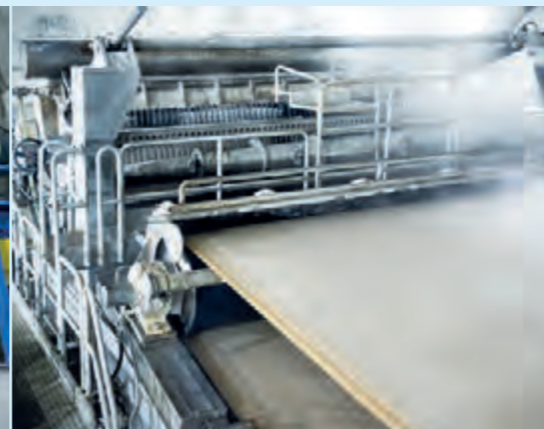
▲ PrimeLine™ tissue machine. In 2012 alone, four 50,000 t/a ANDRITZ machines started up at Hengan's Chongqing and Jinjiang mills. Four additional machines are on order.
