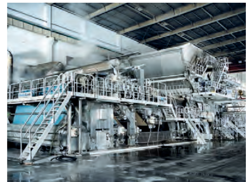
▲ Hengan's PrimeLine™ machines are equipped with the latest resource-saving technologies: the PrimeDry Steel Yankee and the ReEvaporation system.
