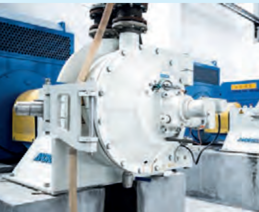
▲ ANDRITZ Double Disc TwinFlo Refiner for optimum fiber development.
