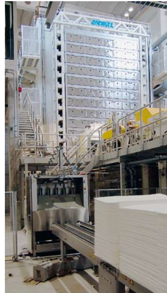
▲ No other pulp company has a product range that includes euca pulp as well as strong reinforcement pulp. The main markets for Botnia's FRB Euca pulp are China and Europe. Approximately 70% will be sold to Botnia's owners (UPM-Kymmene and M-Real) and approximately 30% as market pulp. As part of the drying plant delivery, Andritz supplied two Andritz dryers, two Cutter/Layboys and four automated baling lines.
